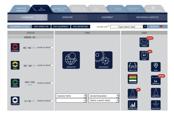
The Dashboard provides an overview of the current status of all equipment for the selected analysis type and included a number of different functions that allow you to view data, records, reports and manage your equipment.
