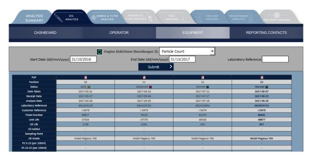
When viewing an individual piece of equipment click the **Data** button to view the tabular analysis data. You can use the drop-down box at the top of the page to view pre-defined groupings of tests/elements as well as create graphs and download using the Export button.
