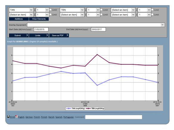
The graph function allows you to plot the trends of analysis for individual equipment for a selection of tests/elements. Select the criteria required and press the **Submit** button to generate the graph. There are quick links for **additives** and **wear elements** are provided and the individual tests or elements can be scaled using each **individual multiplier**.
